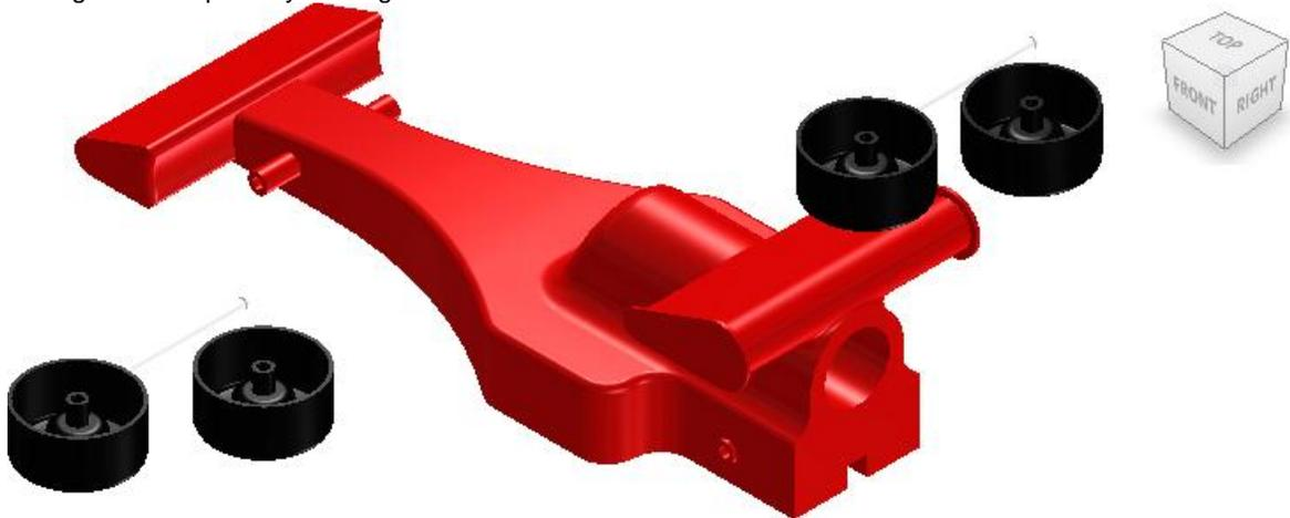
8) Move a wheel closer to the front left wheel extension and zoom into this area.
