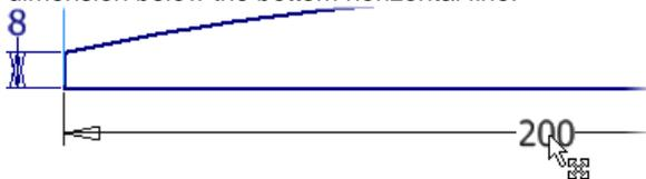
9) The sketch dimensions are parametric, meaning that the value of the dimension controls the size of the geometry. Change the size of the 200 mm by double-clicking on it and enter **250** in the Edit Dimension dialog box and then press Enter or click the green check mark in the dialog box.
